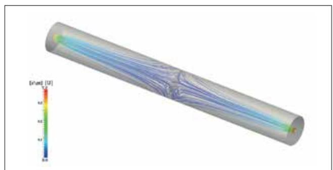
CFD-calculated fluid path while back-pulsing
