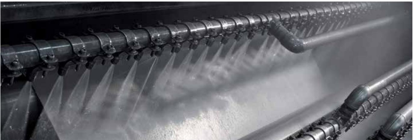
To provide our premium sand screens without any signs of dirt is a necessity as well. Dirt, dust and oil might still remain on the surface of wires after the weaving process. Therefore GKD has several continuous cleaning devices in place which use the power of ultra-sonic.
