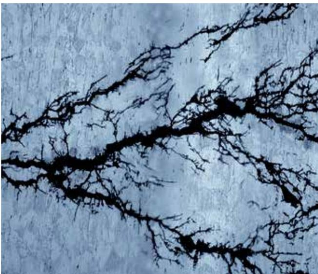
*Stress corrosion Cracking (SCC)*
