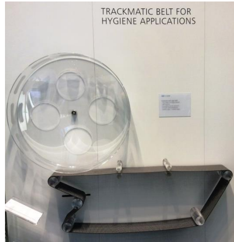
Picture 1-2: The GKD business unit WEAVE IN MOTION presented ultra-flexible, self-tracking woven metal belts and innovative belt coatings.
