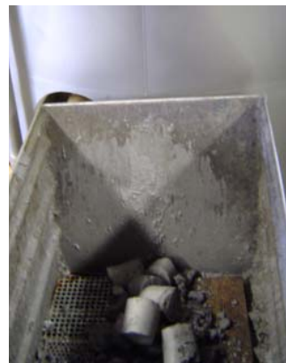
Picture 5: The compressed, dry briquets are collected in the briquet wagon.
