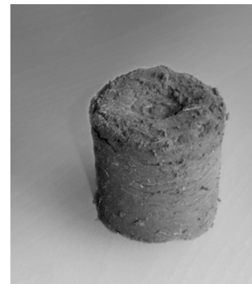
Picture 6: Compressed filter sludge in the form of an easy-to-dispose briquet.
