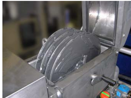
Picture 2: Inside view of MAXFLOW with deposited filter sludge.
