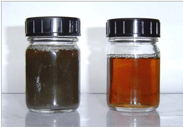
Picture 4: Contaminated cooling lubricant oil from the grinding works (left) and cleaned cooling lubricant oil after filtration with MAXFLOW (right).
